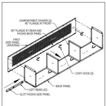
**Step 3:** Attach the second top shelf, the second bottom shelf, and an additional three coat hooks to the second back panel as in step 1.
